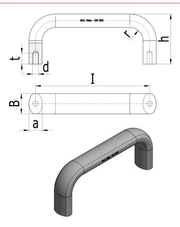
$\begin{array}{lll} a & = 17 \\ b & = 26 \\ d & = M8 \\ h & = 57 \\ I & = 300 \\ r & = 17 \\ t & = 12 \\ Weight in (g) = 445 \\ \end{array}$
